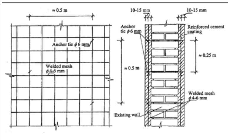
Figure 14: Seismic-strengthening by reinforced cement coating (WHE Report 73, Slovenia)
