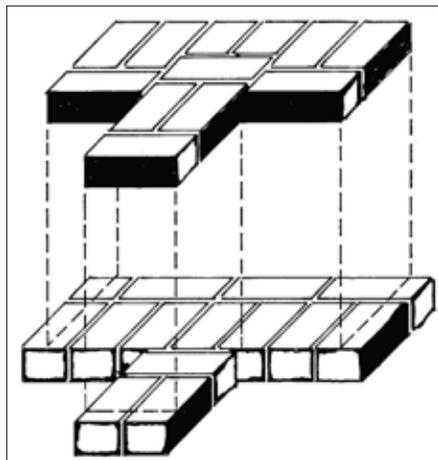
Figure 6: Details of bonding arrangement for masonry units at wall junction (WHE Report 73, Slovenia)
